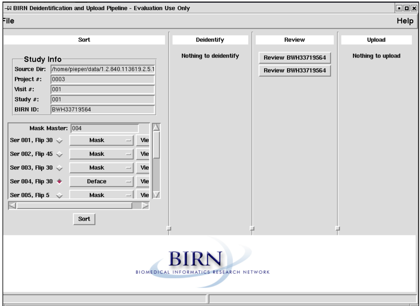
Figure 1. Main interface to the BIRNDUP pipeline. The four panels correspond to the four main steps requiring user intervention in the deidentification and upload process.
