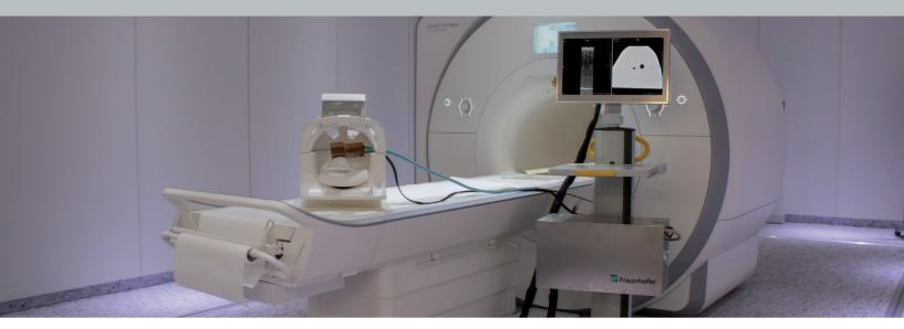
MR-compatible ultrasound research platform for multimodal imaging and a combination of the advantages of MR imaging and ultrasound imaging for ultrasound-supported movement tracking of internal organs during MRT imaging.
