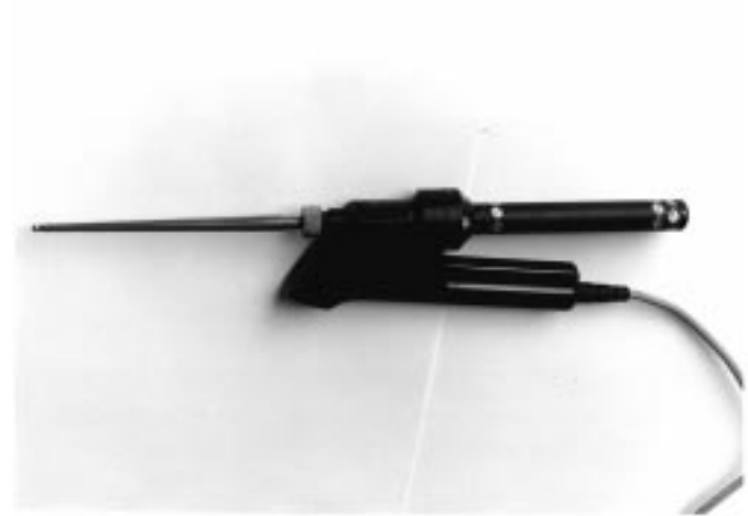
Fig. 4. Photograph of probe and probe attachment. The probe attachment is approximately 15-cm long and consists of a thermoplastic handle equipped with two pushbutton controls and an anodized aluminum housing containing an array of 19 IRED's. The identity of the tool and the configuration (relative position and orientation) of the rigid-body array of IRED's are stored in a chip at the end of the cable that connects the tool to the system. Marker localization is performed using a 10.5-cm-long probe constructed of anodized titanium alloy that tapers down to form a 3-mm-diameter spherical ball at its distal tip (shown). Surgical navigation is performed using a 13-cm-long probe with a 1.5-mm-diameter spherical tip (not shown).
