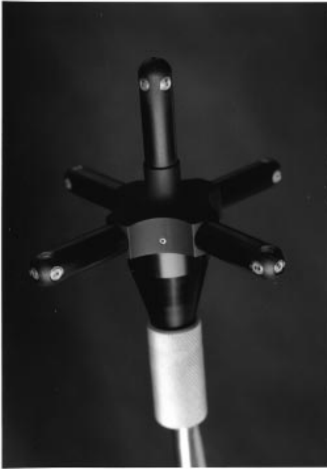
Fig. 5. Photograph of reference emitter. The reference emitter consists of five arms that form a 3-D cross containing an array of 20 IRED's, four on each of the five arms. The housing is constructed of anodized aluminum alloy. Each arm is approximately 6-cm long. The reference emitter is rigidly attached to the patient's head via a multijointed arm and a Mayfield skull clamp (the head fixation device).
