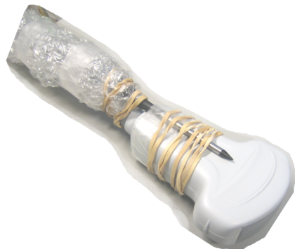
Figure: Ultrasound probe with attached tracking sensor
